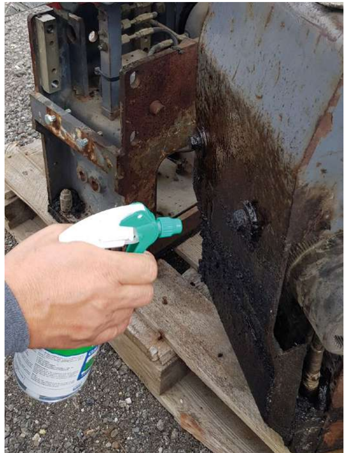
Removing bitumen with GS 200
