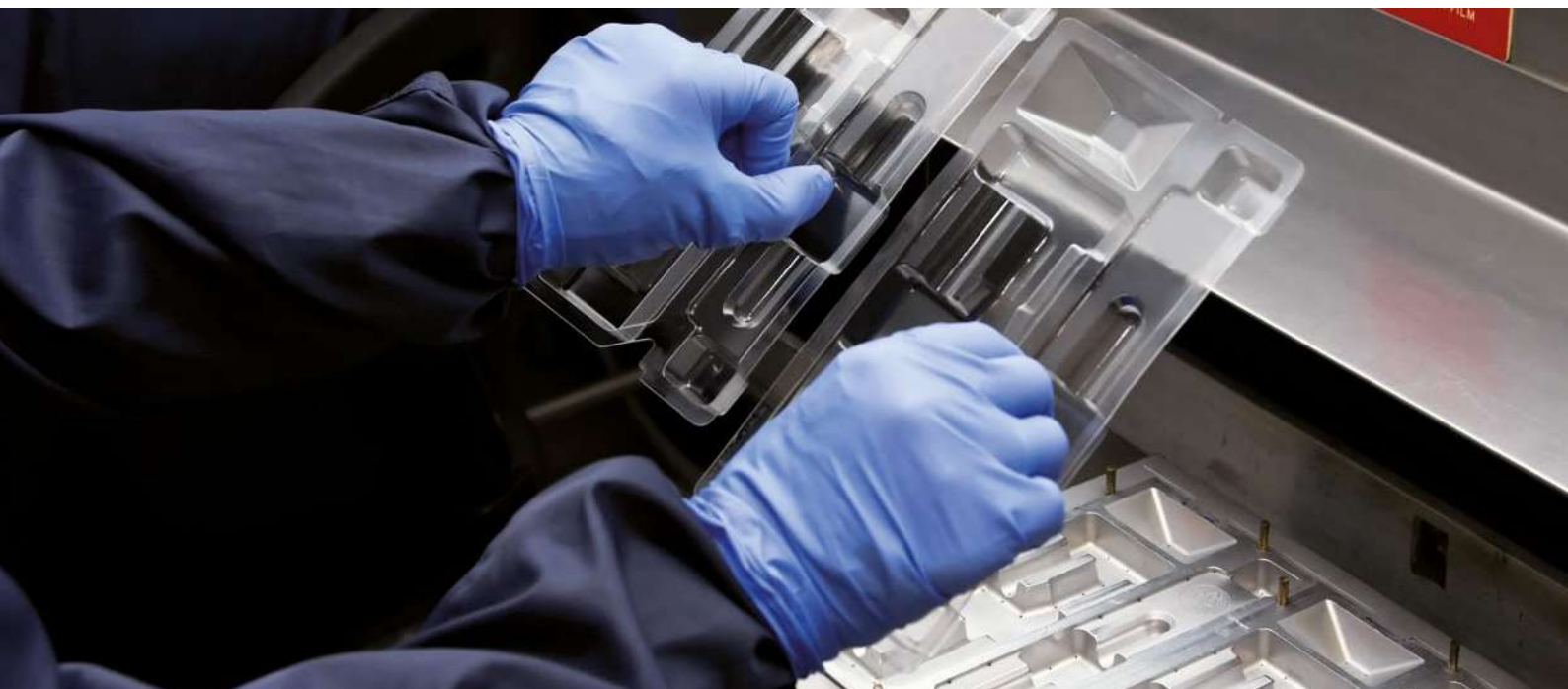
Use of FT in the plastics industry – cleaning of plastic injection moulds
