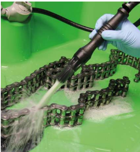
Cleaning oil-contaminated parts in the BIO-CIRCLE GT-i
