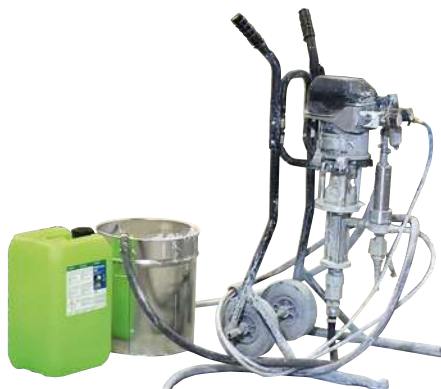
Hose system cleaning with PROLAQ Liquid
